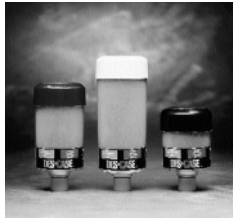
HYGROSCOPIC BREATHERS FOR HYDRAULIC RESERVOIRS INCLUDE COLOR-CHANGE VISUAL INDICATORS THAT SIGNAL WHEN DESICCANT IS SATURATED.
