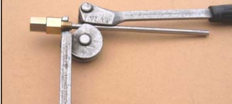
Bend the Pitot Tube & Disassemble
