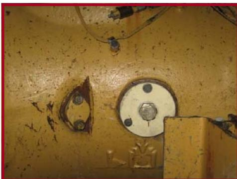
Proper orientation of the down tube inside the differential after installation is essential. Metal to metal contact between the cover plate and the plug & sampling valve, will insure the position of the down tube, relative to the cover, plate when it is installed. It is necessary to specify the bolt hole location on the cover plate, ( i.e. 3 bolts, 4.25" BC, 1 bolt at 12 o'clock).
