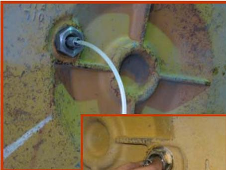
For the **OILMISER™ (Severe Duty) Plug & Sampling Valve**, only the immediate area must be wiped clean. Removing the sealed Steel Hex Cap, presents a large open cavity, with a clean Hi-Flow Sampling valve (SV-HF25) easily accessible. The sampling probe (SP-HF25), with a short length of sampling tube and vacuum pump quickly attaches by hand to the sampling valve. The oil sample is drawn, and the Steel Hex Cap is reinstalled. Job done, time, 15 minutes or less.
