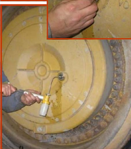
The **OILMISER™ (Severe Duty) Plug & Sampling Valve**
