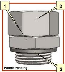
The OILMISER™ PSV-PT includes a plated steel threaded hex plug (1), a plated steel hex cap (2) and a bonded rubber plug seal (3). The steel hex cap mates with a raised threaded boss (4). When the hex cap is fully engaged on the hex plug, a captive O’ring (5) seals the steel body & cap against any outside contamination getting inside the machine.
