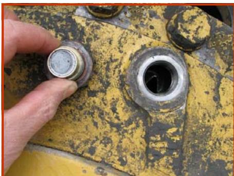
In the absence of oil cleanliness data that would accrue from a running series of oil analysis reports, all lubrication and hydraulic oils are discarded and replaced with new oil at the 2000 hour Service, Maintenance & Overhaul schedule.
