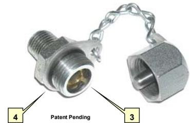
When the oil sample has been drawn with a vacuum pump, the plastic sampling tube or the **OILMISER™** pass-thru probe is withdrawn. The tube seal/wiper strips any residual lubricating oil from the outside surface of the sampling tube, leaving it virtually free of any oil film. Without the need for the
