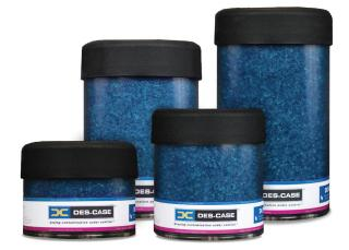
The Des-Case EX-series breather combines offers a high flow rate and extended life from check valves. As wet, contaminated air is drawn through the unit, multiple 3-micron polyester filter elements remove solid particulate, and color-indicating silica gel extracts moisture. When air is expelled from the container, the top foam pad prevents oil mist from contacting silica gel or entering the atmosphere.
