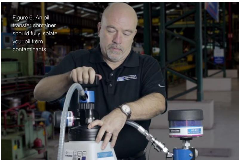
Figure 6. An oil transfer container should fully isolate your oil from contaminants
