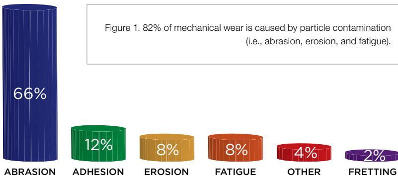
Figure 1. 82% of mechanical wear is caused by particle contamination (i.e., abrasion, erosion, and fatigue).
