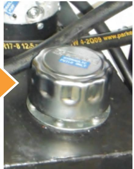
⚡ **Hydraulic breathers and fill ports should be modified to include high efficiency desiccant breathers.**
