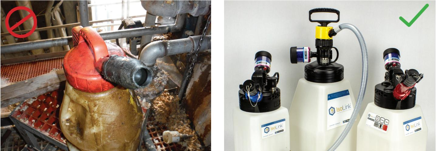
Figure 4 - the transfer container on the left has been left open and the lid has to be removed to fill it. The container on the right is completely sealed and can be filled using quick connects
