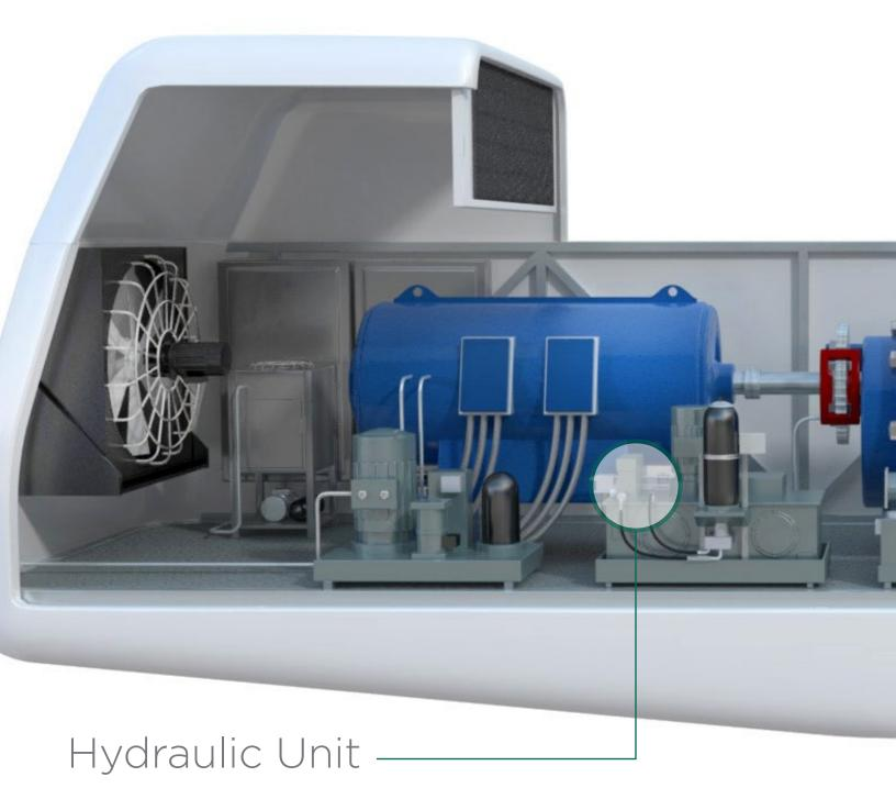
The turbines use a hydraulic system that provides a braking mechanism for a unit, but can also be used for hydraulic pitch control on the blades. The oil in this application not only transmits power, but it also provides lubrication, heat transfer, and transports contaminants to be filtered out.
