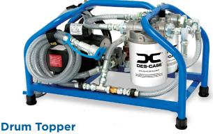
When oil is going to be stored in drums, this compact, portable and lightweight filtration system can be used for filtering new oil directly from the drum, filling transfer containers and can act as an offline filter for up-tower equipment.
